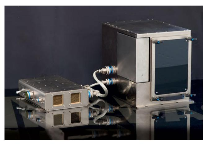
A specially modified 3D printer could fabricate spare parts and construction blocks.
